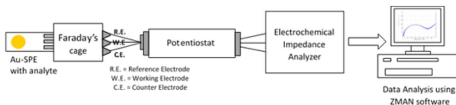
**Figure 1.** Block diagram of the electrochemical impedance spectroscopy instrumentation system.
